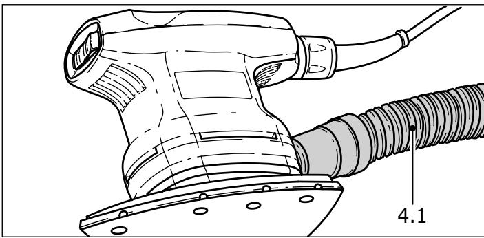
In this case, the extraction pipe ( $\varnothing$  27 mm) (4.1) of the extraction unit is connected to the suction nozzle.
